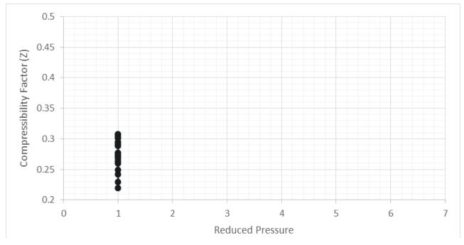
Fig. 2. Compressibility factor vs reduced pressure at critical state showing Nelson-Obert characteristics
